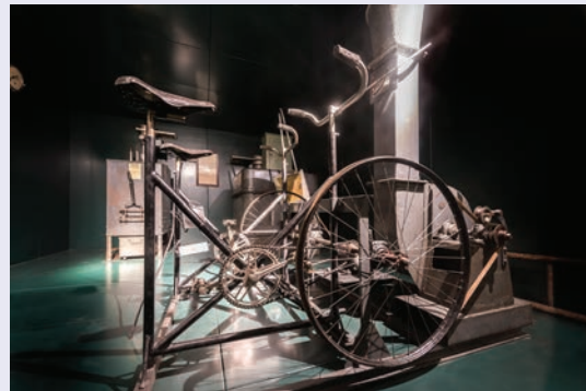
A bicycle generator in the shelter supplied electricity and filtered air © Pierre Antoine
